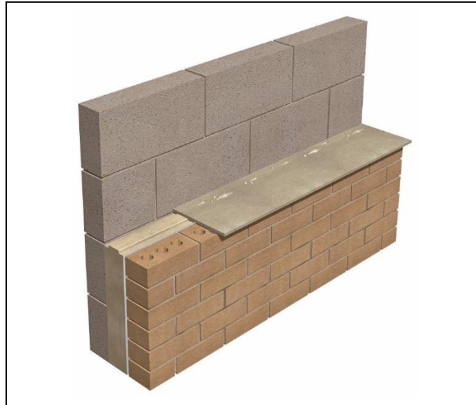
Figure 4 Use of cavity board when cleaning off excess mortar
