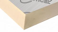
Eurothane GP is a thermal insulation board. Its core consists of rigid polyisocyanurate PIR foam. The board is faced with a gas diffusion tight multilayer foil on both sides. Grid pattern on both sides.
